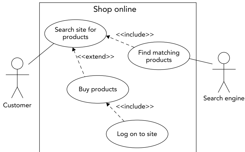
FIGURE 5-11: A use case diagram shows actors and the tasks they perform (possibly with subtasks and extensions).
